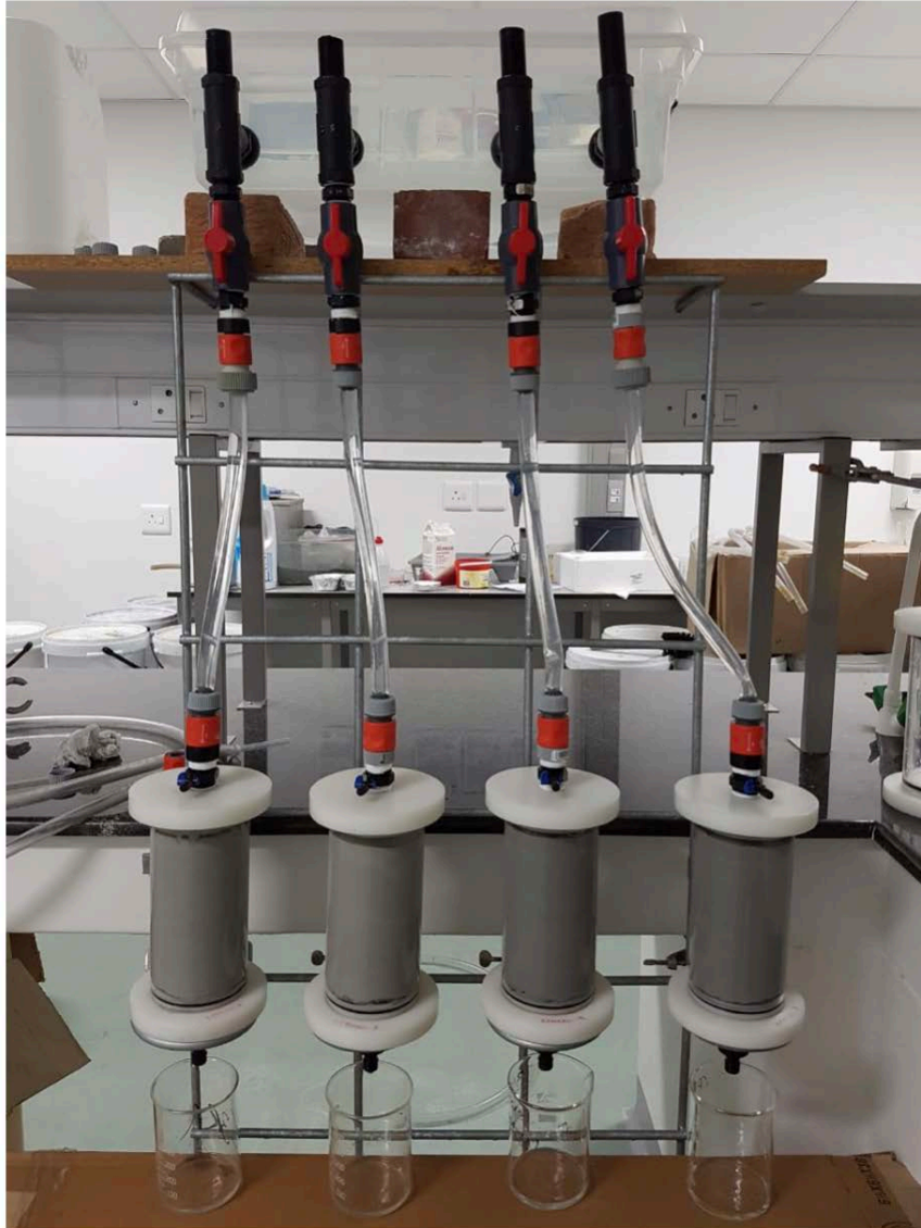
Figure 5. Acid mine drainage neutralization testing
