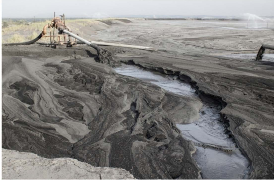
Figure 1. Dumping fly ash in ponds
