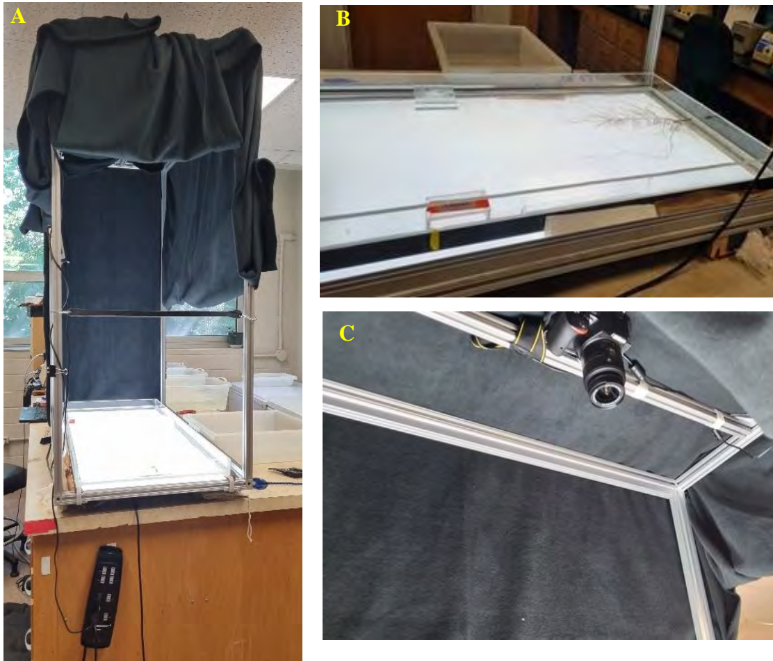
Figure 3. Photos displaying root image analysis in the lab. Note: photo booth (A), tray with soybean root for image capturing (B), and cabled Nikon camera for image taking (C).
